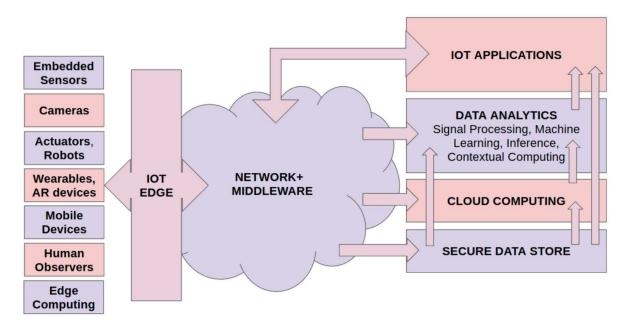
Figure 1. Typical IoT System Architecture
